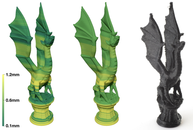
Fig. 9. Distribution of the maximum allowable structuring element size suggested by our algorithm. Left-to-right: corrected models obtained using varying structuring element size range of [0.1, 1.2]mm , [0.6, 1.2]mm and the corresponding printed model.
