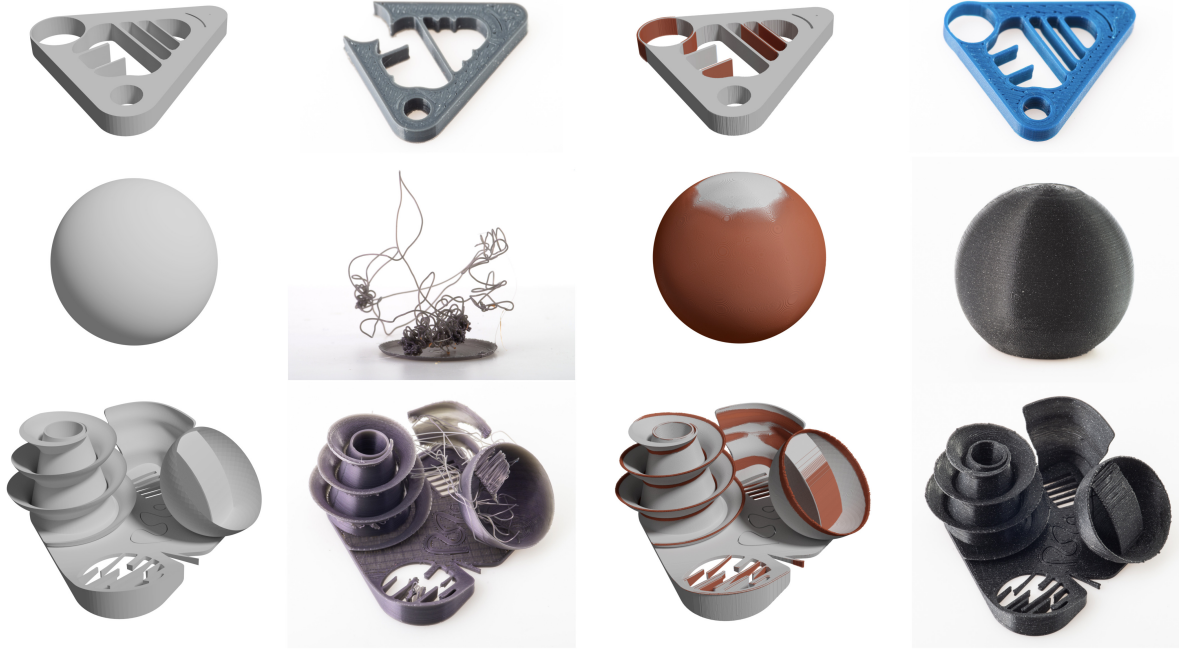
Fig. 7. Model correction results. Left-to-right: input uncorrected models with their corresponding failed prints, corrected models and their successful prints. Added and removed material are highlighted in red and blue, respectively.
