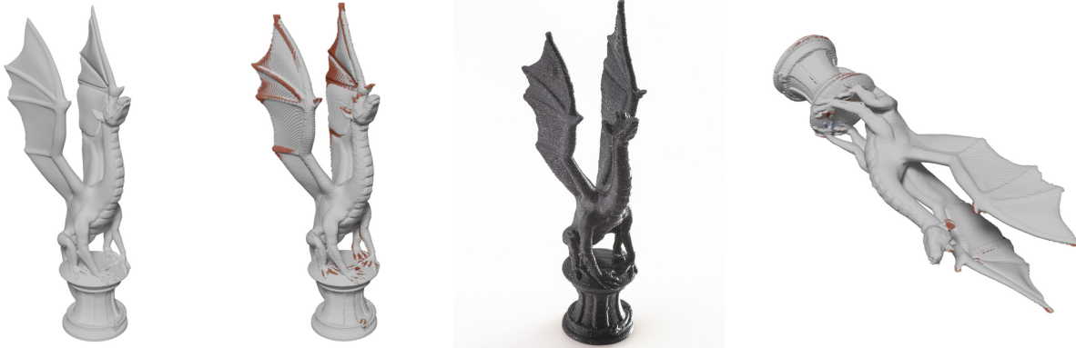
Fig. 1. We present a method for correcting 3D models to make them manufacturable with the intended additive manufacturing process. Our approach analyzes the input model (gray) layer by layer and provides modifications to the shape (in the form of addition (red) or removal (blue) of material) to avoid fabrication errors due to the minimum printable feature size. Required modifications are minimized by optimizing the build direction (right).
