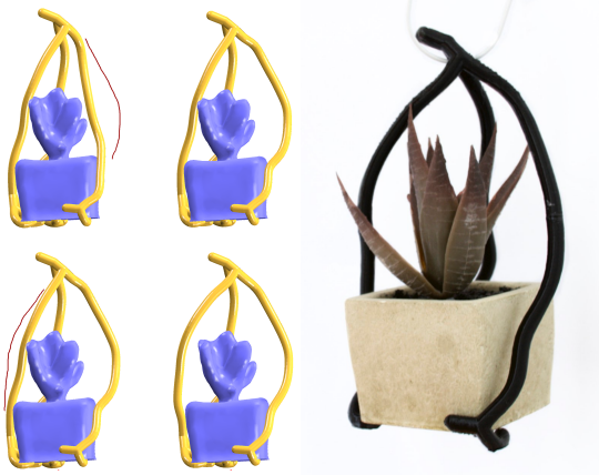
Fig. 9. Use of sketch modifications for a functional purpose. Top part of the planter holder is enlarged to be able to insert the planter. Left: Sketch modification steps, Right: 3D printed result with the inserted planter.
