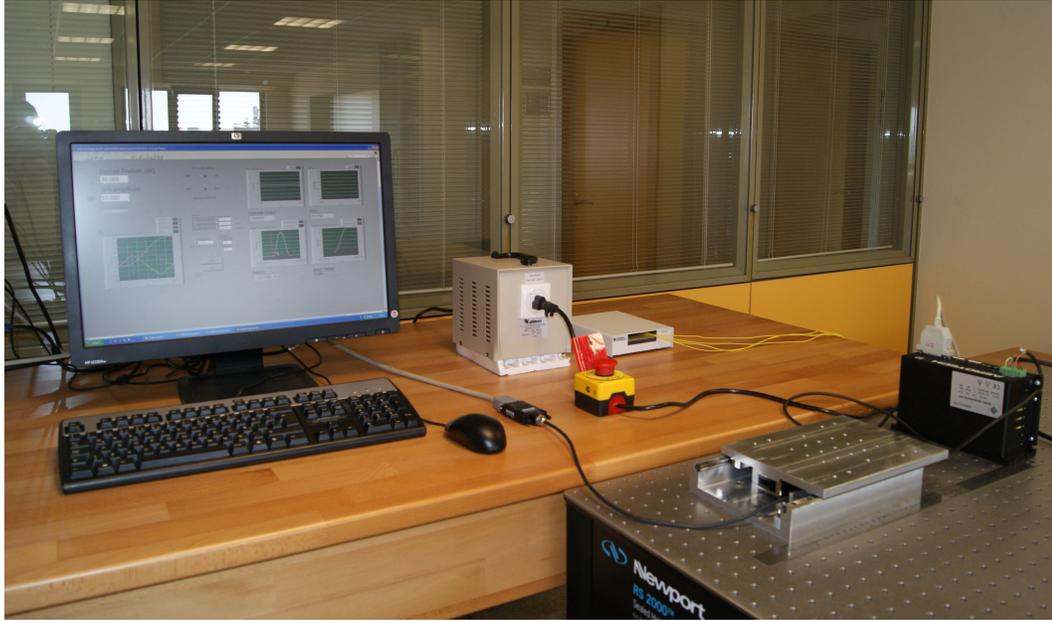
Figure 2.3: Photograph of testbed for the single-axis slider system
